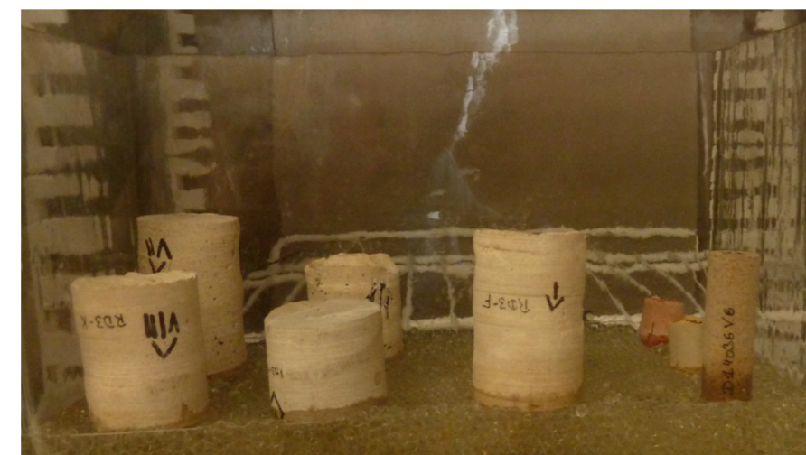
Fig.5 : Lithium silicate impregnation
