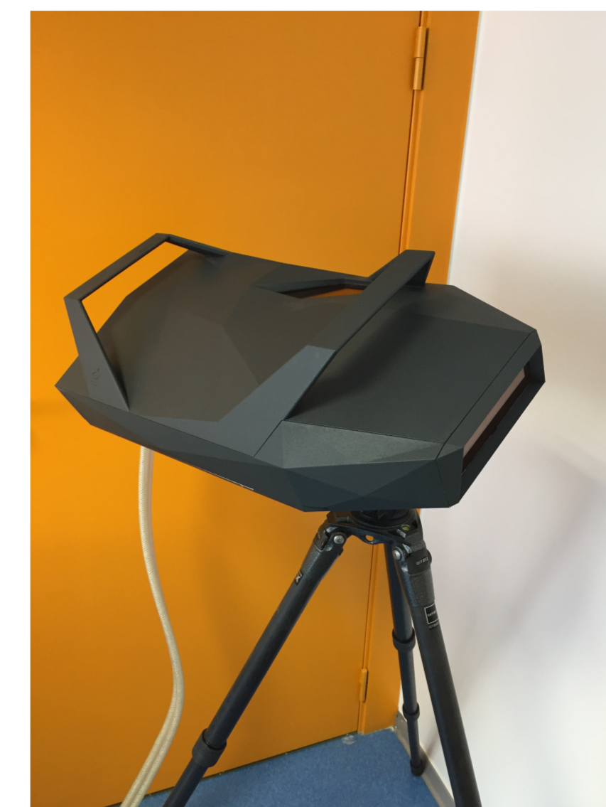
Fig.2 : Portable LIBS system used by Epitopos
