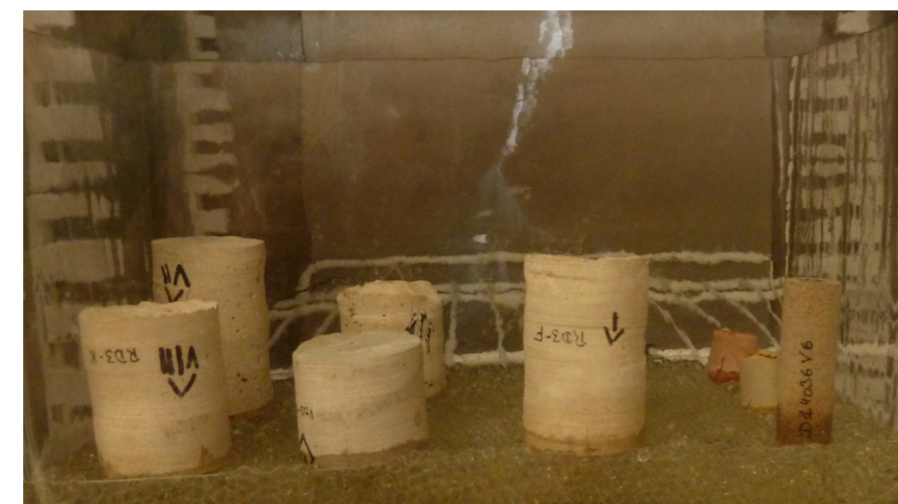
Fig.5 : Lithium silicate impregnation
